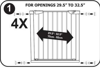
1. Insert part (E) as shown on all four corners of the gate. (Make sure flat end faces gate.)
