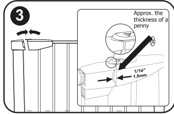
For smooth gate operation, make sure gate is level and the latch gap is only 1/16" (penny width). NOTE: Too loose or tight will cause latch to not function properly.
