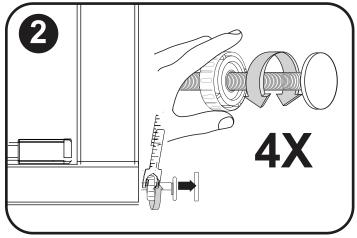
With gate sitting on floor, twist to secure gate in opening. If needed, use wrench **(F)** to tighten.
