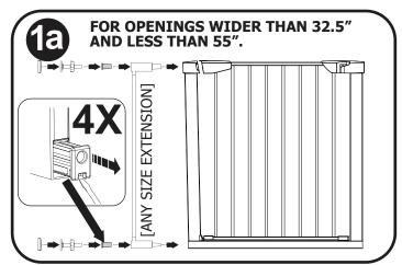
Remove standard inserts on all four corners. Put extension inserts into gate tubing and then put standard inserts into extension, then part (E).
