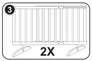
3. Slip feet onto bottom of gate.
