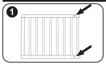
**1.** Loosen screws on gate (**2X**).
