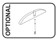
To permanently attach foot to gate, attach with screw.
