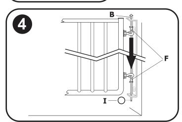
Hang gate by inserting hinge rod (**B**), through top of mounted hinge bracket (**A**), through upper plastic shoulder washer (**F**), through both eye bolts, through lower plastic shoulder washer (F), and finally through bottom of hinge bracket. To sécure hinge, insert key ring (I) through hole in end of hinge rod. Gate can be mounted at angles up to 30 degrees.
