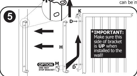
Mount latch assembly (**K**) to gate using 3/4" bolts with serrated washers (**D**). Attach wall mount for latch assembly (**H**) up into part (**K**) that is now secure on gate. Slide gate out to mark holes for (**H**) on attaching wall. (\*OPTIONAL ONE WAY 5. BRACKET INSTALLED HERE) Then attach the wall mount of latch assembly to wall using Phillips head screws (**C**). Optional long screws (**J**) maybe be used to attach gate to stud through dry wall.
