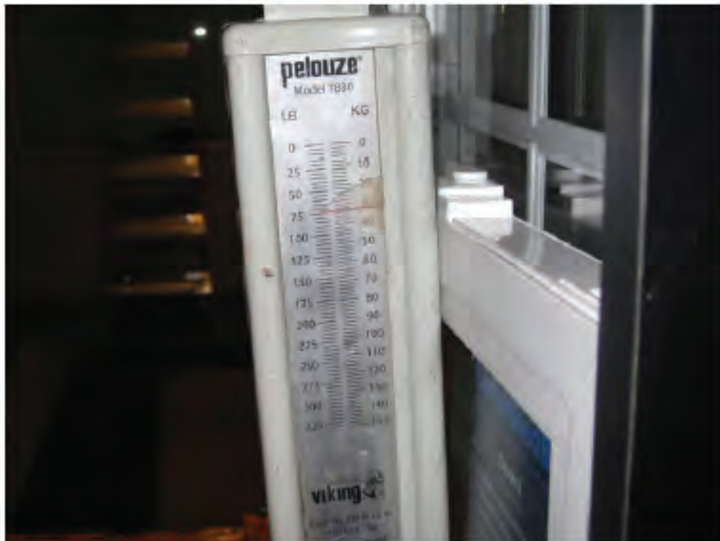
Photo No. 6 View of Window While Under 75 lbf Load No.1
