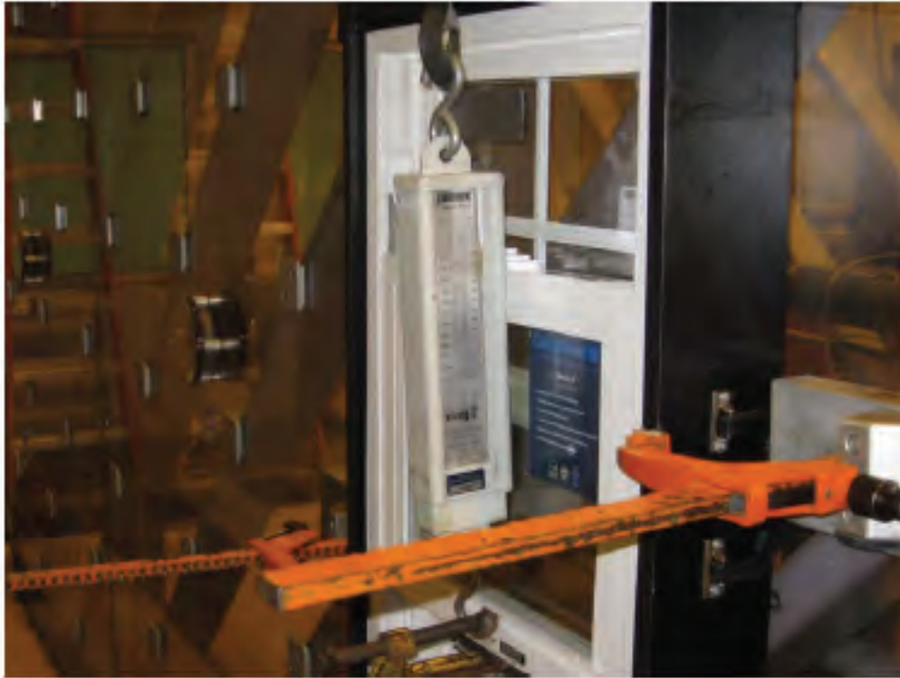
Photo No. 7 View of Window While Under 75 lbf Load No.2
