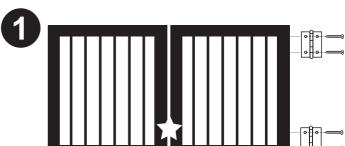
Gate panels are mortised for extra hinges. Simply install extension by adding two (2) hinges with screws.
